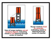
The Front Range (**FR**) panel or light is usually lower than the rear range (**RR**) panel or light. Each range provides a mariner with a given lateral sensitivity at a given distance from the near end of the channel. Lateral sensitivity is expressed as <u>Cross-Track Factor</u> and lends a more physical feel to the performance of the range.
